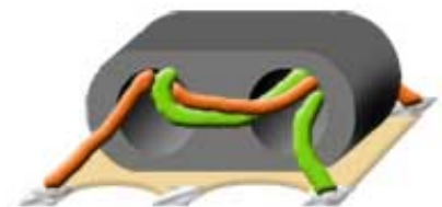
Fig 11.5.2 Surface Mount VHF Transformer.
